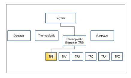
THERMOLAST<sup>®</sup> K stands for versatile TPE compounds. The middle block between the polystyrene domains makes the TPE a soft, elastic material. This formulation allows use of the Thermoplastic Elastomers in diverse areas of application.
