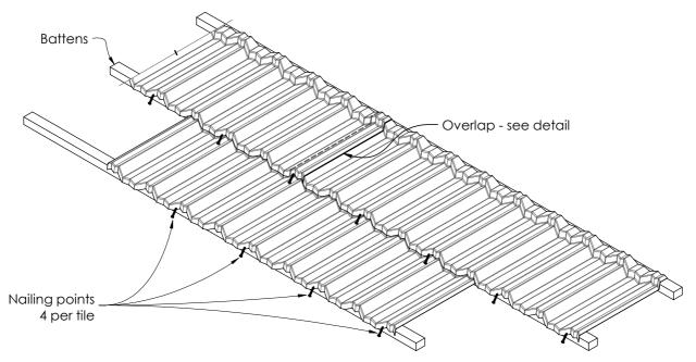
Figure 4.2 Nailing Detail
