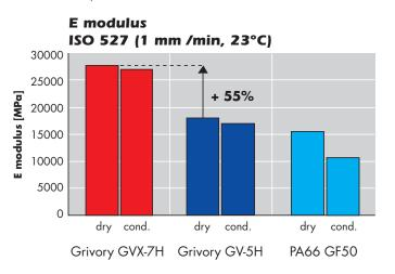
Grivory GVX-7H exhibits an E-modulus which is up to 55% higher than that of Grivory GV-5H. This is a valid comparison since Grivory GVX-7H has comparable flow properties and can therefore be processed similarly to Grivory GV with 50% glass fibre reinforcement. Surface quality and warpage are also best in class, making Grivory GVX products ideal for high-quality metal replacement and, in particular, for very stiff, thinwalled, complex components with long flow paths.
