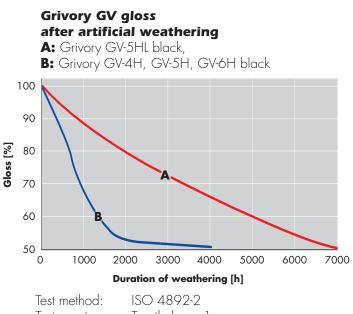
Test specimens: Tensile bars, 1 mm Criterion: Gloss (60) in % of the original value
