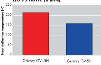
Heat deflection temperature ISO 75 HDT/C (8 MPa) The three-dimensional fibre-felt structure gives the matrix additional stability. This results in enhanced mechanical performance, especially at higher temperatures. This improved performance is clearly visible in the stresselongation diagram as per ISO 527.
