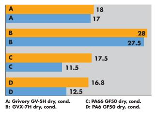
Grivory GV is positioned in the range of high quality engineering plastics. As a rule, Grivory GV has the characteristic properties of polyamides. In direct comparison with traditional materials based on polyamide 6 (PA6) or polyamide 66 (PA66), Grivory GV is characterised by the fact that, unlike most polyamides, its mechanical properties are hardly affected by the absorption of moisture. Stiffness and strength values remain at a high level.
