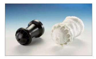
The fibre-felt structure increases the resistance to cracking and prevents cracks from spreading much more effectively than materials reinforced with short glass fibres. In an impact penetration test, the test plate is not punctured. Instead it shows an area with hinge fractures.
