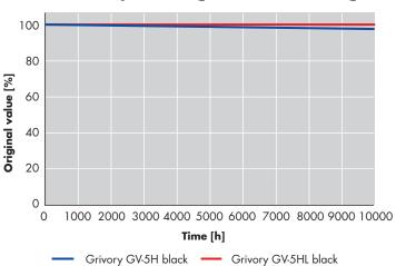
Tensile impact strength after weathering
