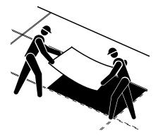
Where Servipak boards abut the parapet, pipe bays or abutments they should be pre-measured, and accurately cut to size by incising with a sharp knife and breaking on edge. The joints between the Servipak boards should be dry and primed with Primer B2.
