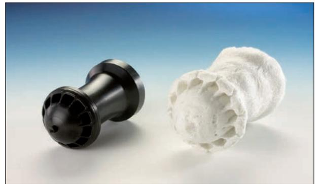
The fibre-felt structure increases the resistance to cracking and prevents cracks from spreading much more effectively than materials reinforced with short glass fibres. In an impact penetration test, the test plate is not punctured. Instead it shows an area with hinge fractures.
