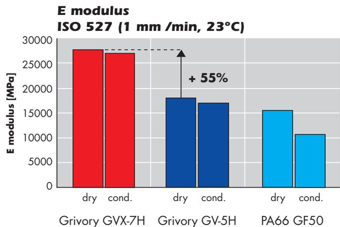
Grivory GVX-7H exhibits an E-modulus which is up to 55% higher than that of Grivory GV-5H. This is a valid comparison since Grivory GVX-7H has comparable flow properties and can therefore be processed similarly to Grivory GV with 50% glass fibre reinforcement. Surface quality and warpage are also best in class, making Grivory GVX products ideal for high-quality metal replacement and, in particular, for very stiff, thin-walled, complex components with long flow paths.
