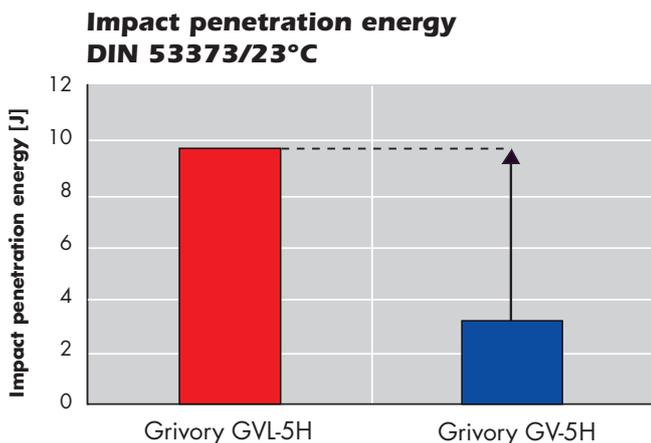
This can be attributed to the structure of the long glass fibres in the component. Unlike short glass fibres, the long glass fibres form a 3-D fibre-felt structure in the component. This becomes visible when a component of this type is pyrolised.
