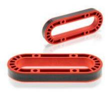
EMS-GRIVORY has now developed endless fibre-reinforced tapes where all fibres are aligned in exactly the direction of the band. The fibres are just as well impregnated as the granules and therefore, exhibit a degree of efficiency on the same level as the theoretically maximum achievable fibre properties. These bands are compatible to the injection-moulding materials used in each case and are welded with the component by being inserted into the mould and over-moulded with the material
