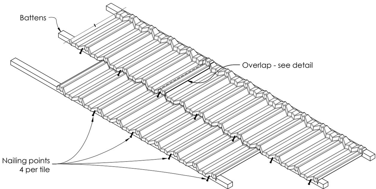
Figure 4.2 Nailing Detail
